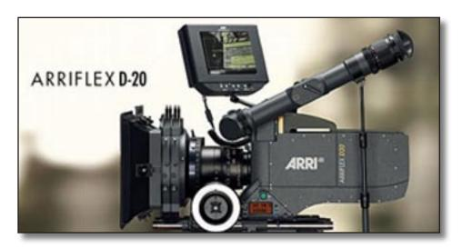
The ARRIFLEX D-20 is a film style digital camera. Because of its single, Super 35-sized CMOS sensor, the D-20 uses the same lenses as 35mm film cameras and has the same depth of field as 35mm film. It has an optical viewfinder, is capable of variable frame rates and is compatible with ARRI film camera accessories. It outputs an HDTV signal in HD mode or via raw sensor information in data mode. See www.arri.com.
